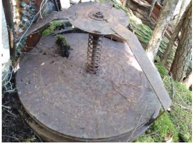
ABOVE: When Bowdrie Widdell first saw the device he took it for a burner used by some backwoods distiller, but his father researched it, and determined it was in fact part of a WWII Japanese Fu-Go, or Fire Balloon. /BOWDRIE WIDDELL. RIGHT: A schematic showing how the Fu-Go was put together.
