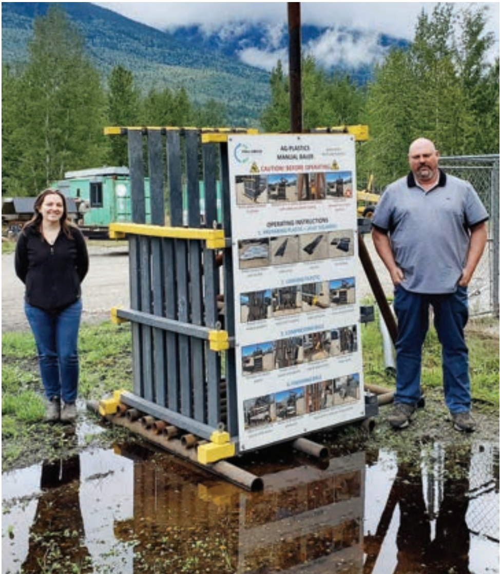
Carly Fraser, Cleanfarms Special Projects Coordinator, and John Peterson, Operations Manager McBride Public Works show off the baler that will help compact and contain large amounts of agriculturally used plastic before shipping. The machine will only be used by appointed and trained individuals. /ANDREA ARNOLD
