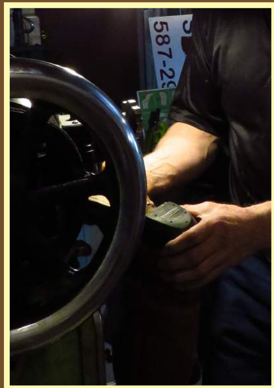
Above: Ryan Vale works on a pair of cowboy boots, using an “outside stitcher” or “C-stitcher.” The machine is used for sewing leather soles onto footwear./ANDREA ARNOLD
